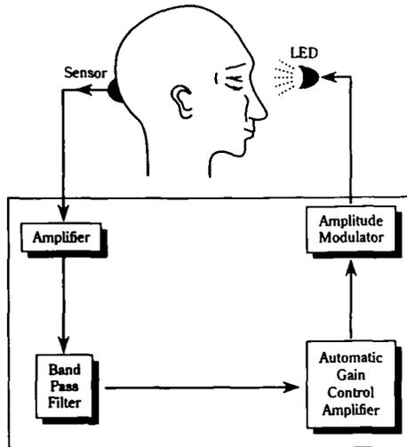
Fig. 1. The block diagram of EEG-driven photic stimulation. LED, light-emitting diodes.
